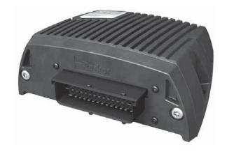
Weight 0.7 Kg -40 to +70 °C Operating temperature Protection outdoor use Voltage supply 11-32 VDC Current consumption (idle) 180 mA (28 VDC) 170 mA (14 VDC) Data interface Parker ICP
