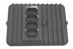
Weight 1.1 kg Temperature range -40 to +85 °C Operating, ambient -40 to +100 °C Storage, ambient Protection outdoor, chassis Voltage supply 9 - 32 Vdc Current consumption (idle) 160 mA (24V) 240 mA (12V) CAN buses **Protocols** Parker ICP (IQAN CAN Protocol) SAE J1939. Generic CAN
