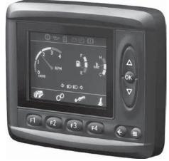
Weight 0.3 Kg -30 to +60 °C Operating temperature -25>LCD off >+75 °C Protection outdoor use Voltage supply 11-32 Vdc Current consumption (idle) 130 mA (28 Vdc) 190 mA (14 Vdc)
